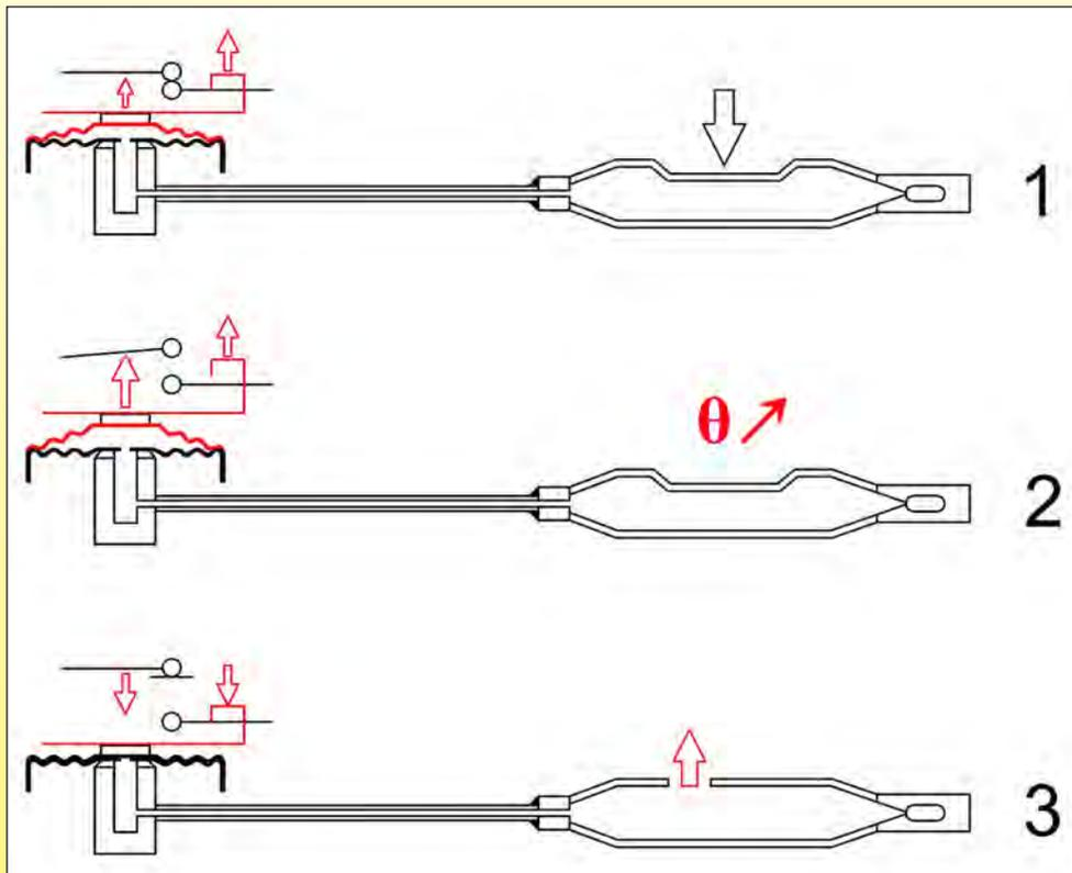
In these systems, after sealing the diastat at ambient temperature, a small bump is made on the bulb, causing an artificial inflation of the bellows (1). It is also possible to produce the same function by sealing the diastat at a negative temperature (-20, -30 °C). By these ways the bellows continues to contract at temperatures below room temperature.
