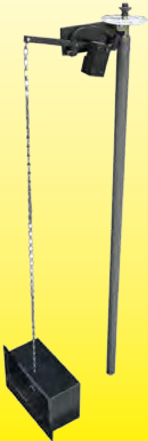
*1788. The first rod thermostat named "Régulateur du feu" invented and built by Jean Simon Bonnemain, French engineer, to control the temperature of a Hatchery in the suburbs of Paris, heated by the first thermosyphon boiler also invented for the occasion.*
