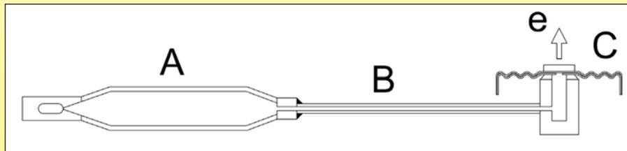
The bulb and capillary thermostats have a closed subassembly called "Diastat".
