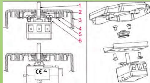
Assembly with back-plate and M4 molded studs (immersion heaters housings)
