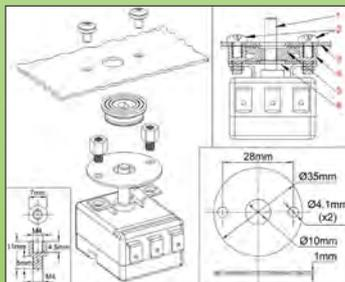
Assembly by 2 holes dia. 4mm, 28 mm distance, with back-plate and M4 spacers
