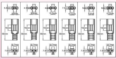
They allow the connection of heating cables on non-heating conventional conductors. When the assembly and filling are performed according to installation instructions, they provide an IP65 seal. Used with AWG15 wires (1.5 mm<sup>2</sup>) FEP insulated 300V, 300mm length (diameter 2.4 mm), equipped with a cable shoe and a tubular crimp terminal. After crimping non-heating wires, the connection to the control box is made with the M20x1.5 accessories with 2.4mm holes.
