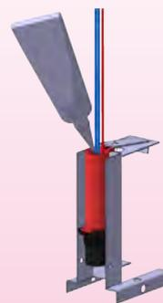
Position the assembly on the filling support and lock it with the upper flap of the sleeve, which has a flange for this purpose. Fill with liquid silicone. It is possible to cut the insertion and filling flaps after polymerization.
