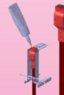
Position the assembly on the filling support and lock it with the upper flap of the sleeve, which has a flange for this purpose. Fill with liquid silicone in the upper shell-hole. It is possible to cut the insertion and filling flaps after polymerization if necessary.
