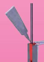
Fill with liquid silicone in the largest neck (connection wires outlet). It is possible to cut the insertion and filling flaps after polymerization.
