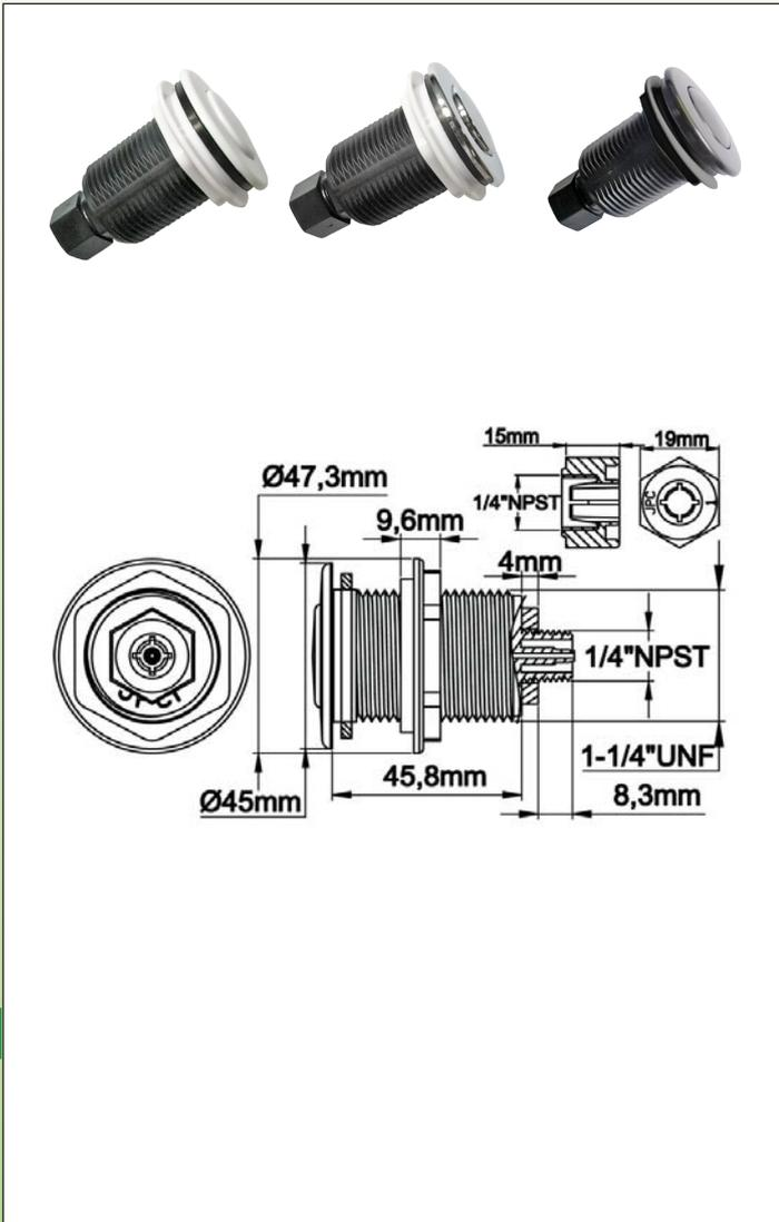
**Use:** Remote operation of air switches. This pneumatic switching technology safely isolates the user from the electrical current. The air transmitters provide the pulse air pressure needed to operate a remote air switch
