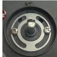
Put the adjustable cam under the thermostat mounting screws. It must be correctly centered. Tighten the 2 screws slightly
