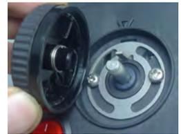
Adjust the cam position to the needed position, tighten the screws, and push the knob on the shaft
