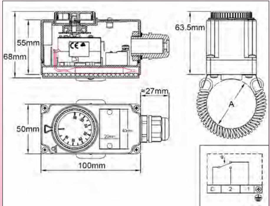
**Housing:** IP65, 100 x 50 x 75 mm, PC-ABS, 20%FG, UL94V0. High impact and UV resistance, with silicone waterproof gasket on thermostat shaft.
