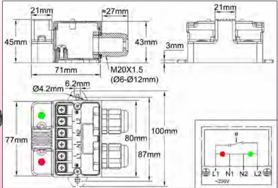
In these boxes, the thermostat, bimetal disc type, is over-molded, and is thermally insulated from the wall on which it is mounted. Its temperature sensing cup is mechanically protected by a grid. It is located in front of the enclosure to be in an area of natural circulation of air.
