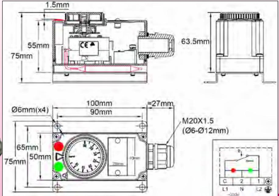
**Housing:** IP65, 100 x 50 x 75 mm, PC-ABS, 20%FG, UL94V0. High impact and UV resistance, with silicone waterproof gasket on thermostat shaft. The SUS304 stainless steel wall mounting plate keeps temperature sensing element away from the wall.
