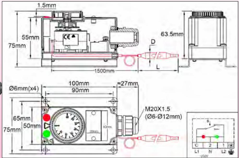
**Housing:** IP65, 100 x 50 x 75 mm, PC-ABS, 20%FG, UL94V0. High impact and UV resistance, with silicone waterproof gasket on thermostat shaft. The SUS304 stainless steel wall mounting plate keeps thermostat housing away from the wall.
