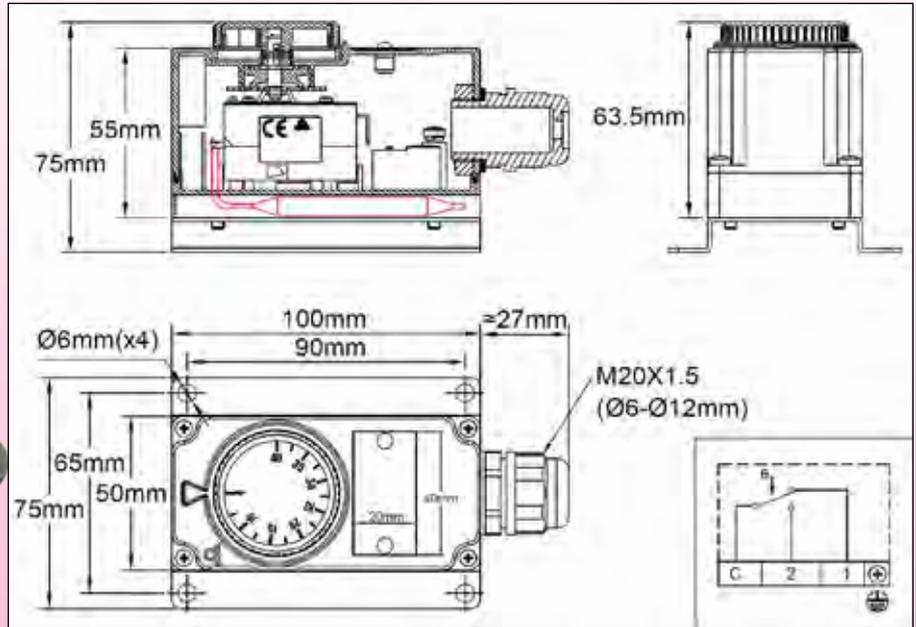
**Housing:** IP65, 100 x 50 x 75 mm, PC-ABS, 20%FG, UL94V0. High impact and UV resistance, with silicone waterproof gasket on thermostat shaft. The SUS304 stainless steel wall mounting plate keeps temperature sensing element away from the wall.
