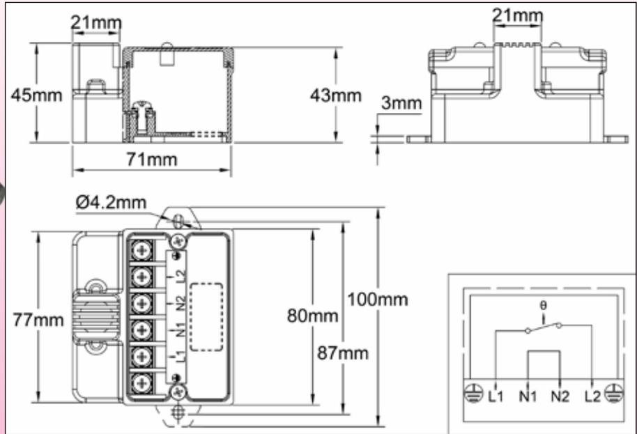
In these boxes, the thermostat is over-molded, and is thermally insulated from the wall on which it is mounted. Its temperature sensing cup is mechanically protected by a grid. It is located in front of the enclosure to be in an area of natural circulation of air. To allow its wall mounting, the box has two outer side lugs, which can be removed when assembly is made with internal screws.
