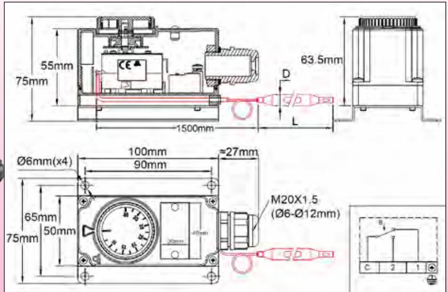
**Housing:** IP65, 100 x 50 x 75 mm, PC-ABS, 20%FG, UL94V0. High impact and UV resistance, with silicone waterproof gasket on thermostat shaft. The SUS304 stainless steel wall mounting plate keeps the thermostat housing away from the wall.
