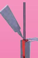
Fill with liquid silicone in the largest neck (connection wires outlet). It is possible to cut the insertion and filling flaps after polymerization.
