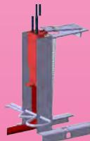
Position the assembly on the filling support and lock it with the flap which has a flange.
