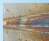
Ending and starting current adjusted correctly
